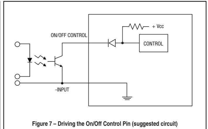
Figure 7 – Driving the On/Off Control Pin (suggested circuit)
