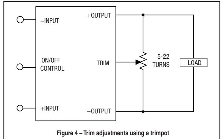
Figure 4 – Trim adjustments using a trimpot
